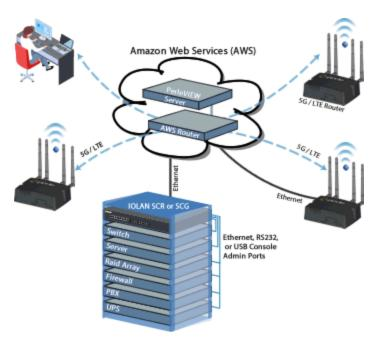
Management ports through Active Standby or Dual Network Access modes. Virtual Router Redundancy Protocol (VRRPv3) enables a group of devices to form a single virtual device to provide network redundancy. The dual AC power supply ensures that console management is available even if the primary AC power source fails. And, protection against electrostatic discharges and power surges is provided with robust 15Kv ESD protection circuitry on each console port.
